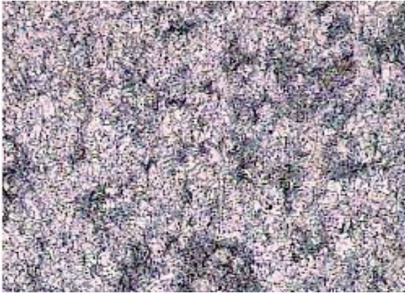
Transversal sample - Spheroidised - Little segregation
