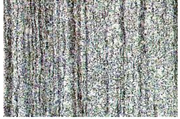
Longitudinal sample – Spheroidised - Strong segregation
